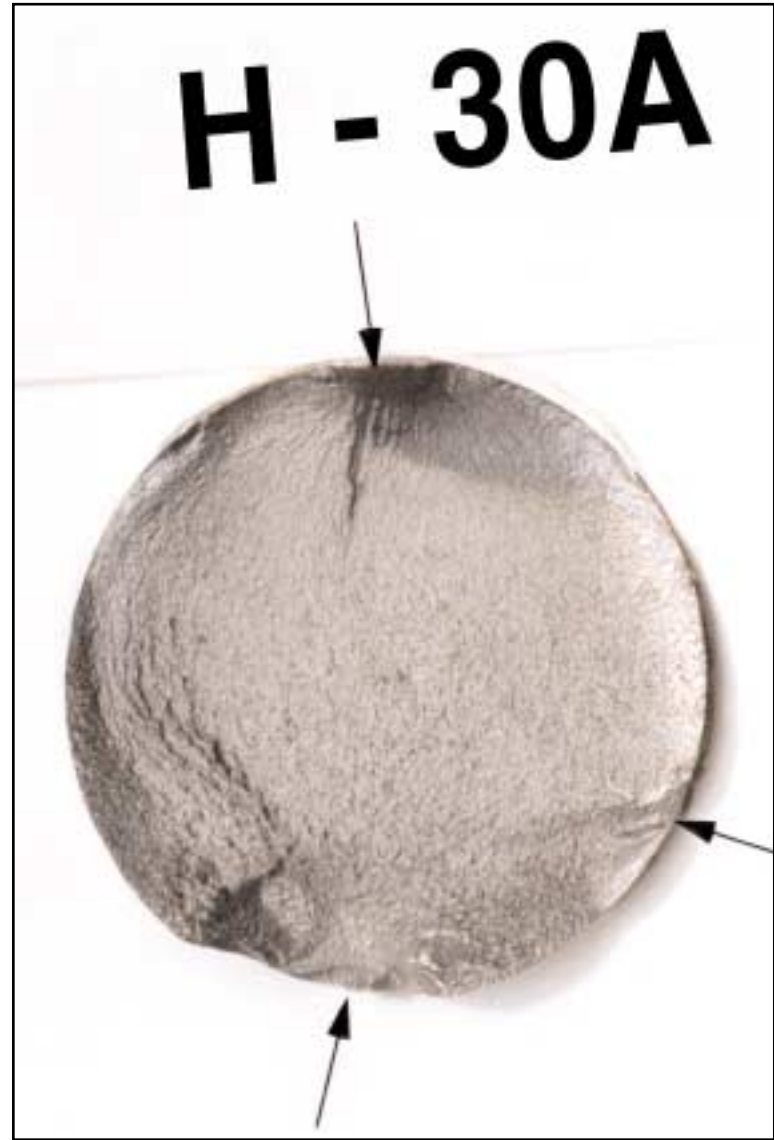
FRACTURED SAMPLE H30A THREE INITIATION SITES
