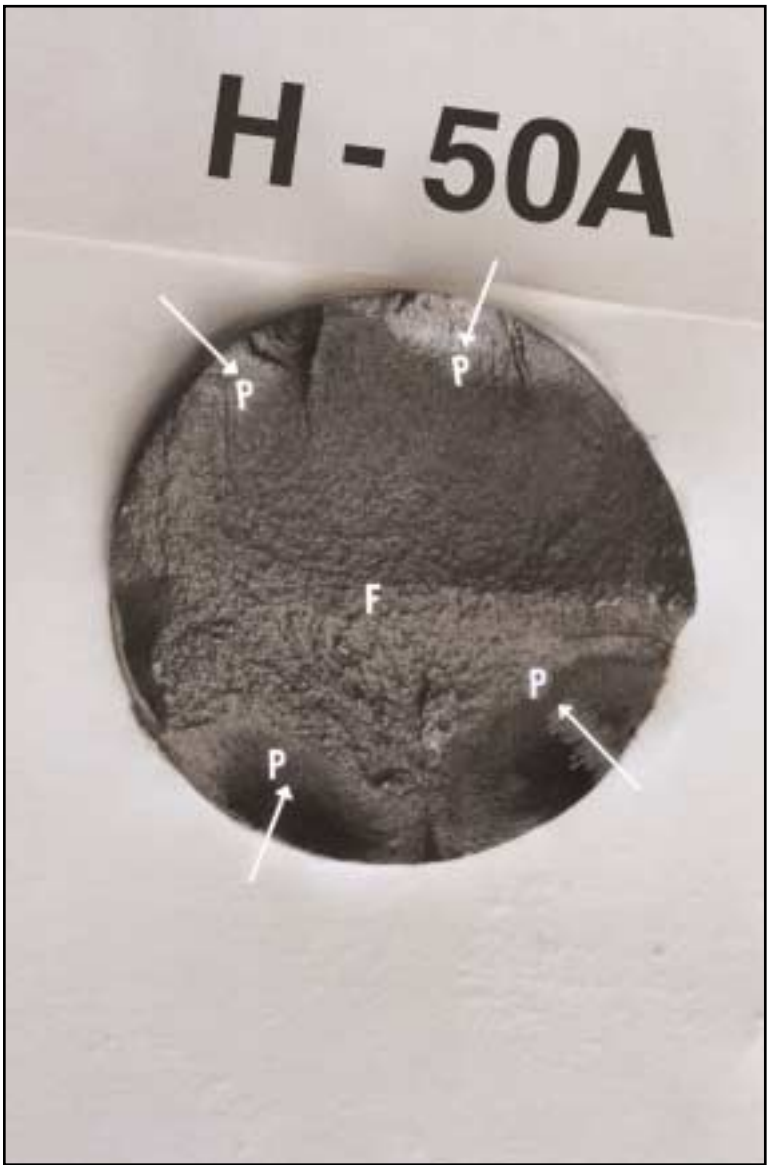
FRACTURED SAMPLE H50A FOUR INITIATION SITES
