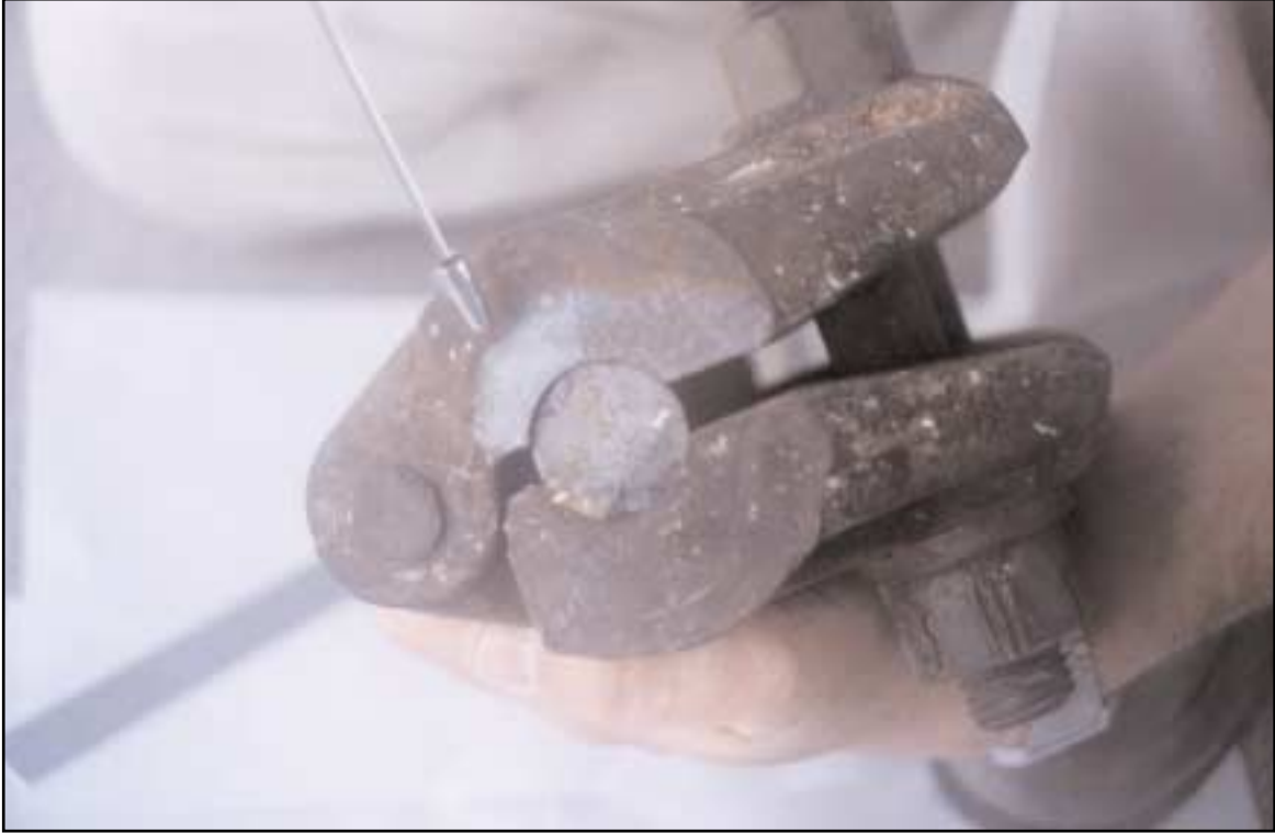
POLISHED ROD FATIGUE FRACTURE INDUCED UNDER ACTUAL FIELD CONDITIONS
