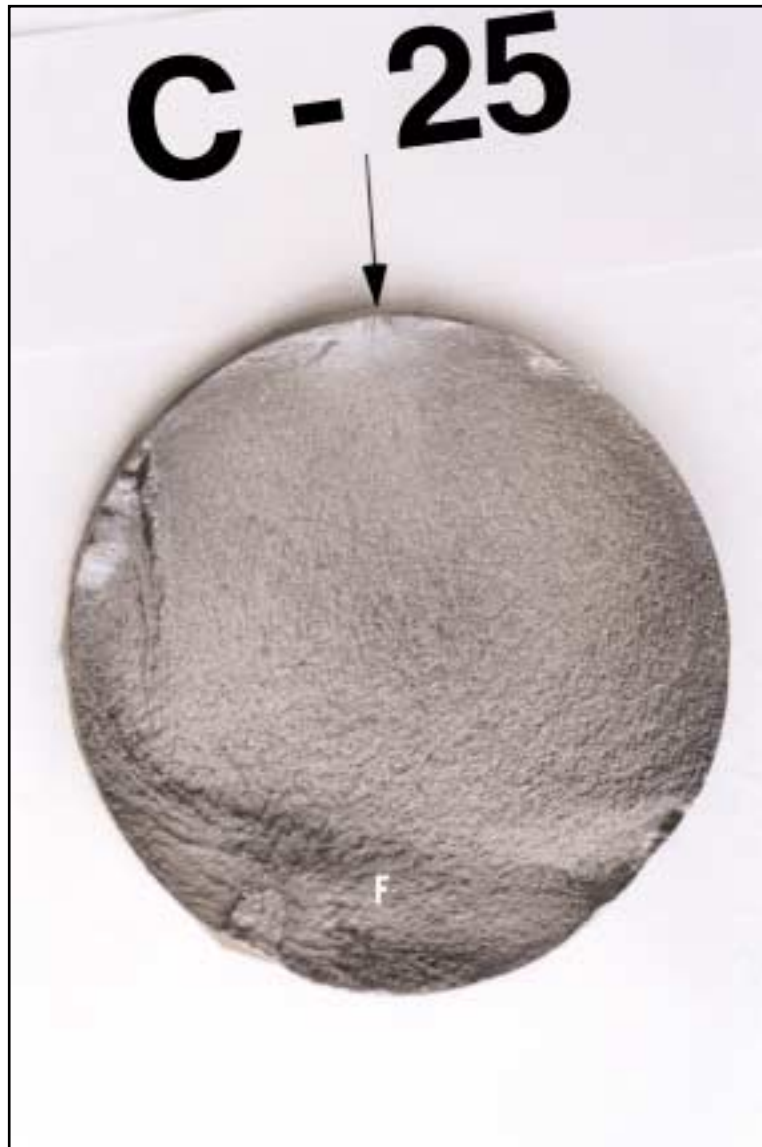
FRACTURED SAMPLE C25 ONE INITIATION SITE
