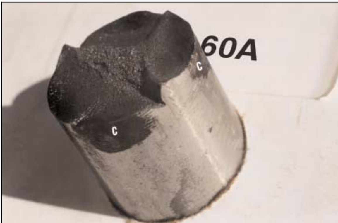
FRACTURED SAMPLE H60A SHOWING WEAR MARKS (DENOTED BY "C")
