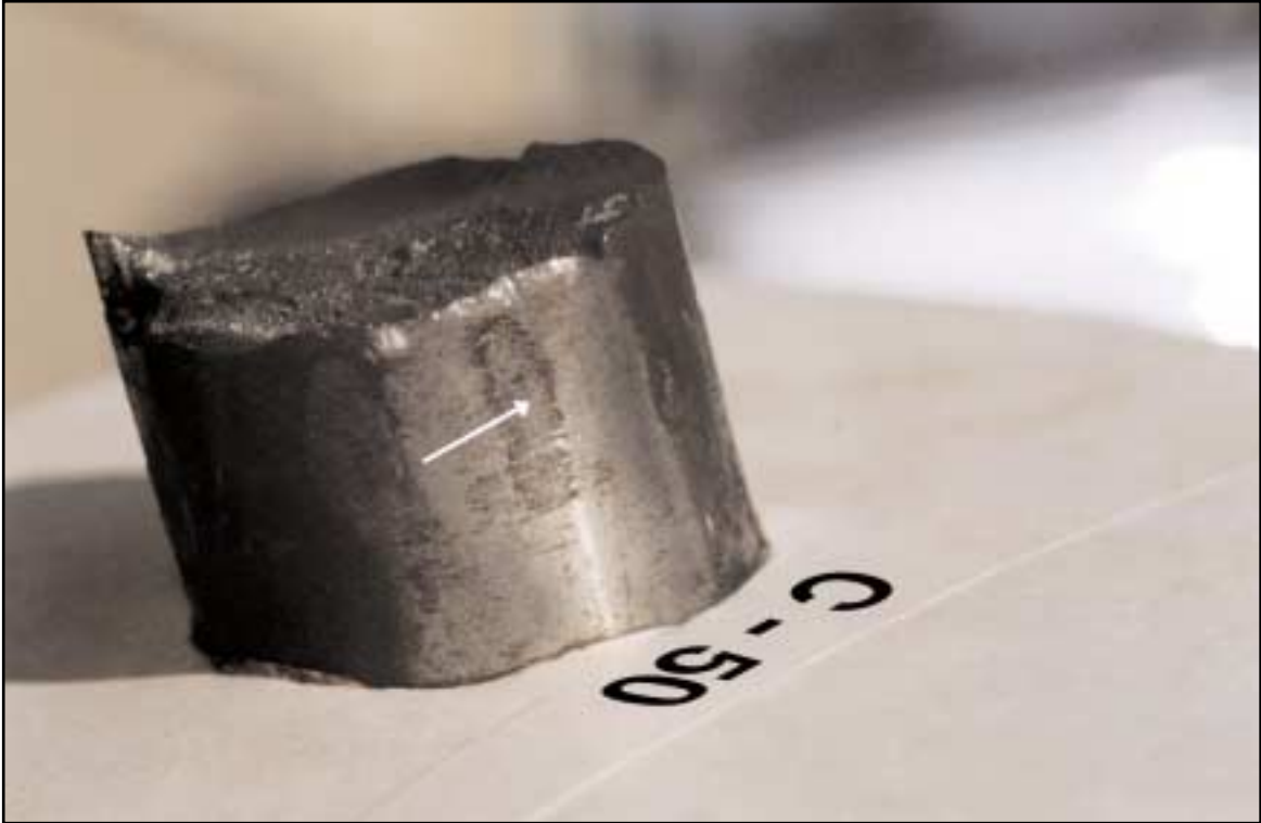
FRACTURED SAMPLE C50 SHOWING WEAR MARK (AT ARROW)
