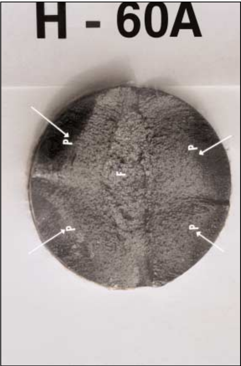
FRACTURED SAMPLE H60A FOUR INITIATION SITES
