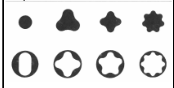
Figure 2 Various Rotor (solid) and Stator Lobe Configurations
